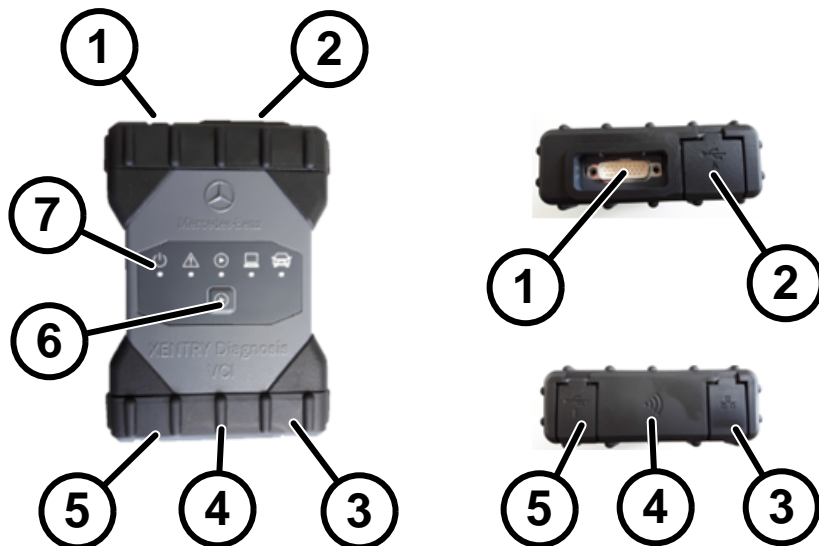
Fig. 41: Conexão do XENTRY Diagnosis VCI
