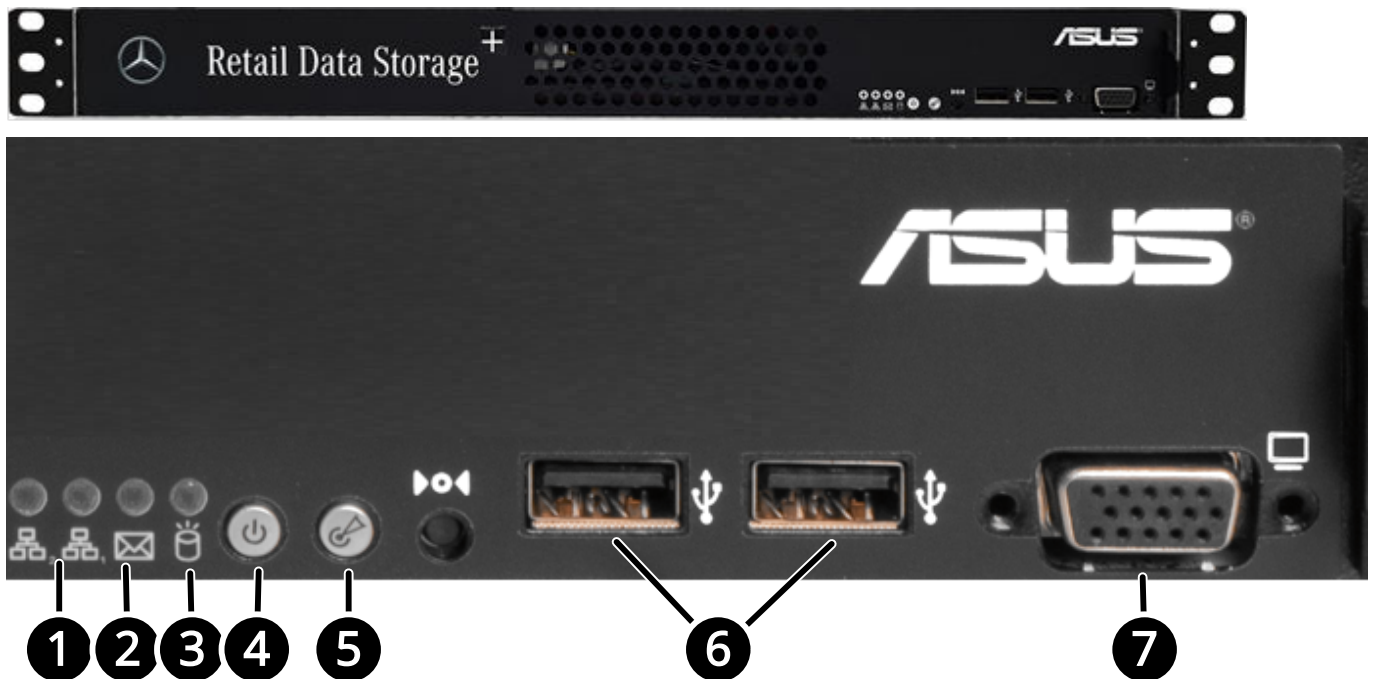
Fig. 50: Retail Data Storage + front view
