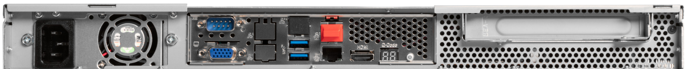
Fig. 6: Rear side with admin port of Retail Data Storage 2
