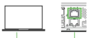
Connect the configuration device to LAN port 1 (temporarily remove the red dust cover).
