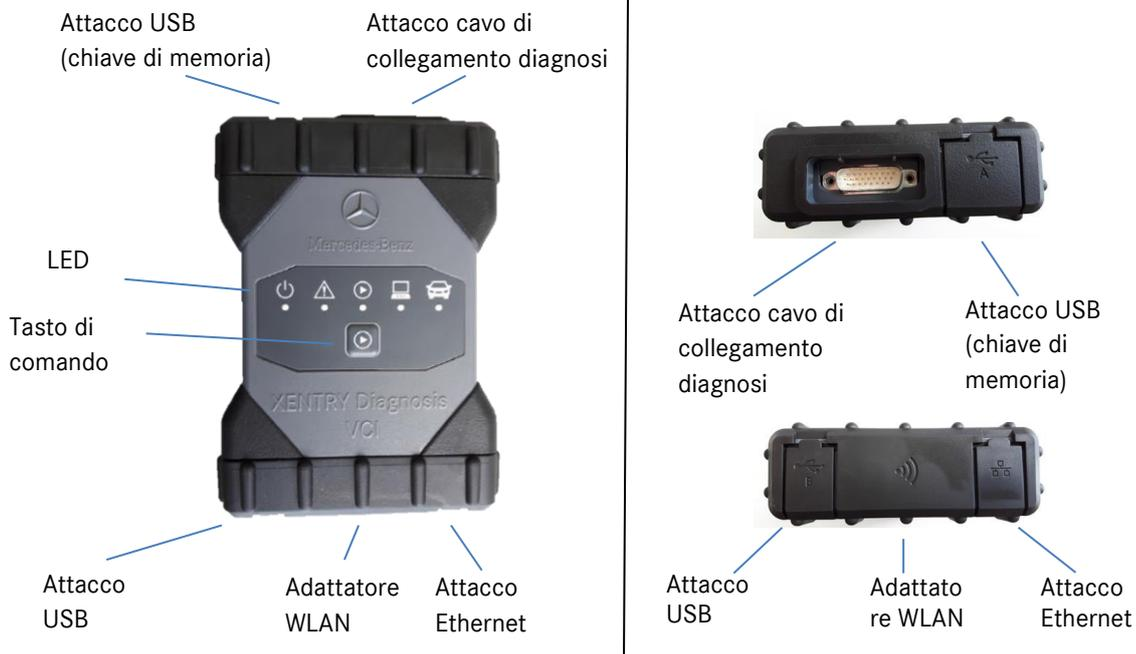
Figura 46: Collegamento XENTRY Diagnosis VCI
