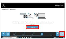
First insert the Wi-Fi stick the diagnosis computer. Connect the VCI to the computer via USB cable and wait for the **beep**.
