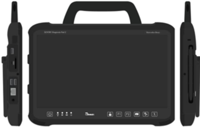
Abb. 39: Anschlüsse XENTRY Diagnosis Pad 2
