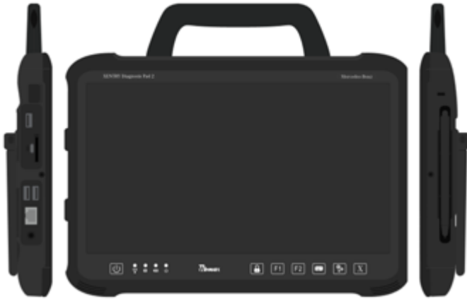
Fig. 39: Connections of XENTRY Diagnosis Pad 2
