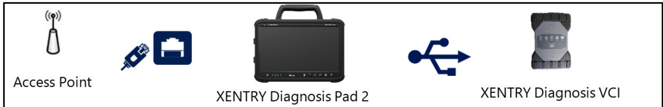
Fig. 20: Connection variant 4: LAN and USB
