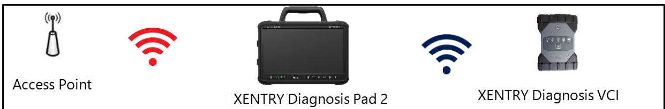
Fig. 17: Connection variant 1: WLAN and WLAN
