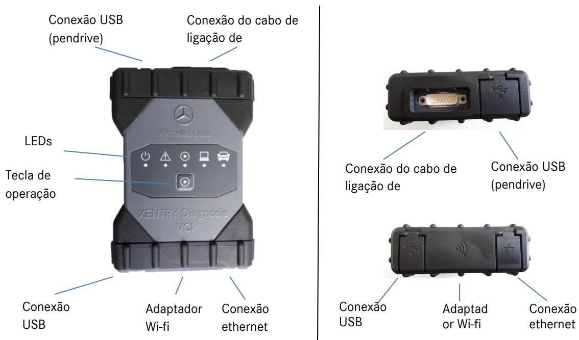
Figura 43: Conexão do XENTRY Diagnosis VCI
