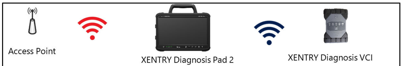
Fig. 17: Connection variant 1: WLAN and WLAN
