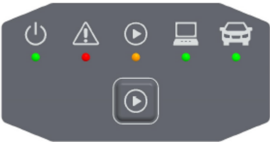
Fig. 42: Status display and control elements on XENTRY Diagnosis VCI
