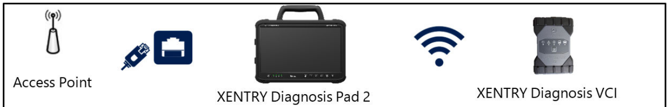
Fig. 19: Connection variant 3: LAN and WLAN
